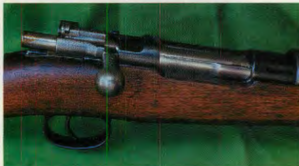
The Model 1895 action is Mauser all the way. Note the length the striker extends from the rear of the striker shroud. This long striker travel is typical for pre-1898 Mauser actions.
